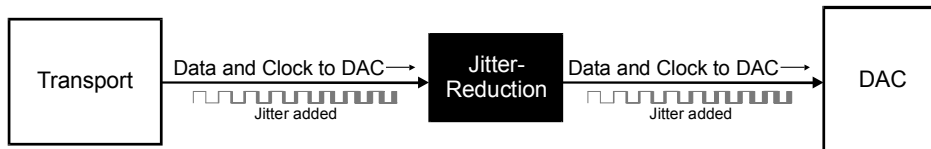
Figure 5. With an outboard jitter-reduction unit, the Clock signal is re-contaminated by the time it reaches the DAC.
