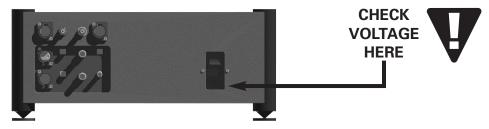
Check to make sure your Wadia S7i CD Player/Decoding Computer has been manufactured for operation at your AC line Voltage. Attempting to use the Player at any voltage other than the specified on the rear of the unit may damage the unit. Damage caused by improper operation is not covered by warranty. If the voltage specified is different from your AC voltage, contact your Wadia dealer.
