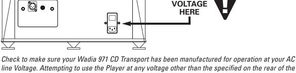
Check to make sure your Wadia 971 CD Transport has been manufactured for operation at your AC line Voltage. Attempting to use the Player at any voltage other than the specified on the rear of the unit may damage the unit. Damage caused by improper operation is not covered by warranty. If the voltage specified is different from your AC voltage, contact your Wadia dealer.
